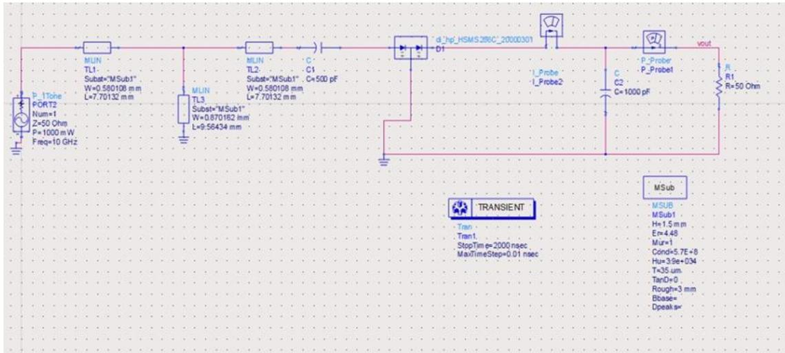
Figure 4: Rectenna Impedance Matching Circuit Topology
